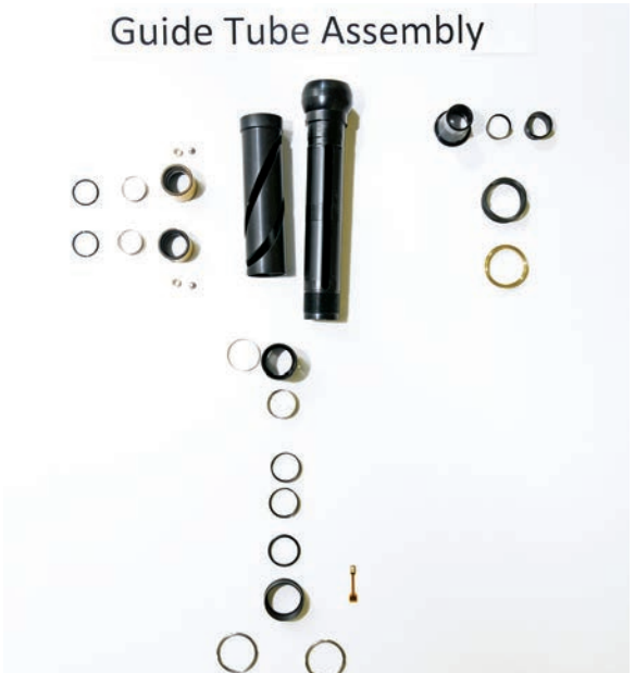
The guide tube assembly is the heart of the scope and contains various lens assemblies providing the change in magnification, the reticle and LED illuminator.
