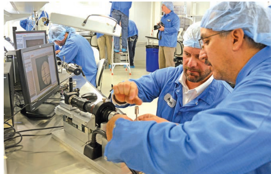
Fortier begins initial assembly of the Steiner's guide tube assembly. Properly cleaning the lenses to the required standard was the hardest part of the job.
